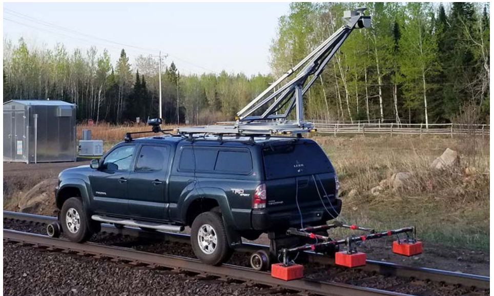
Loram's 400 MHz GPR antenna is able to collect data to a maximum depth of 9 feet. For deeper penetration, Loram deploys lower-frequency antennas such as a 270 MHz antenna as needed, which has a maximum penetration depth of approximately 16 feet.
