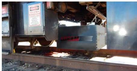
Loram's 400 MHz GPR antenna is able to collect data to a maximum depth of 9 feet. For deeper penetration, Loram deploys lower-frequency antennas such as a 270 MHz antenna as needed, which has a maximum penetration depth of approximately 16 feet.
