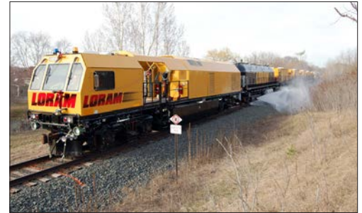
Modular design allows specification of 60–120 grind stones
