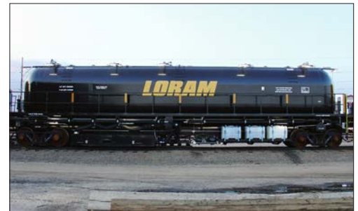
Walk-around water cars offer total capacity up to 75,000 gallons
