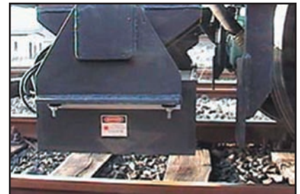
A commonly installed rail profile measurement system compares the rail profile to the desired rail template. Optional grind management software can further recommend optimal machine application.
