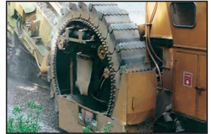
**Digging wheel.** Two digging wheels rip through compacted ballast to a depth of up to 16 inches (400 mm) from the top of the tie. Each wheel is 30 inches (760 mm) wide to allow cleaning from the ends of the ties to the edge of the shoulder.
