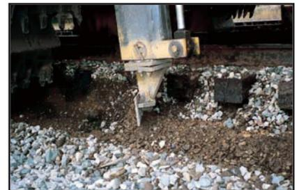
**Scarifier tooth.** A scarifier tooth on each side of the machine undercuts the tie ends up to 5 inches (125 mm) to break up mud pockets and restore drainage.
