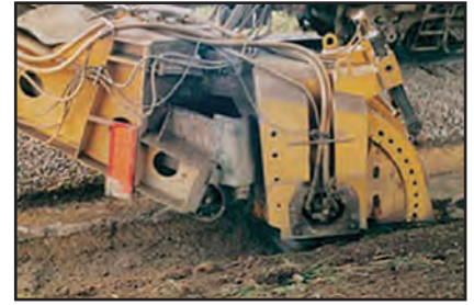
Articulated workhead. The Badger's ditching wheel is mounted on an articulated workhead that can be adjusted to contour the ditch for more efficient drainage.
